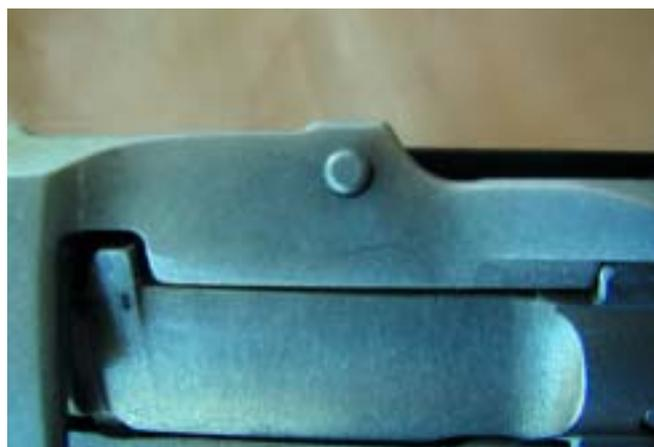
The Mini's bolt hold-open device is a button located on the top left of the receiver.
