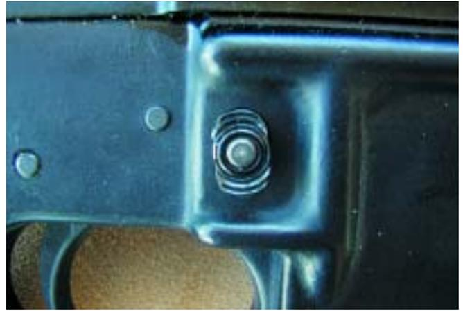
The AR's magazine release is a button located on the right side of the receiver. For speed loads, the author feels this is a better system.
