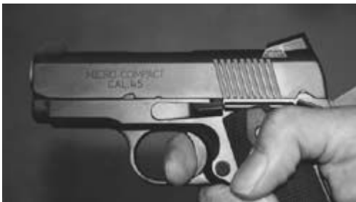
Good ergonomics in action. Short 1911A1 trigger of Springfield Armory Micro Compact allows deep finger placement for good leverage.
