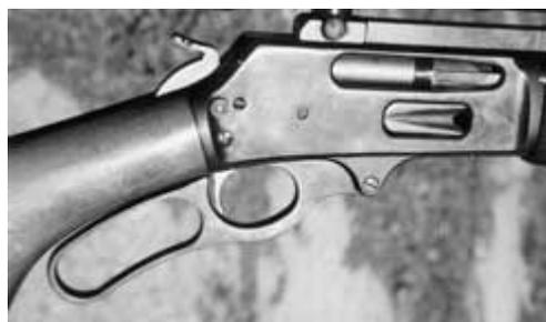
Key Marlin features: side ejection port, traditional loading gate, crossbolt (push button) safety, and extended hammer for easier cocking.
